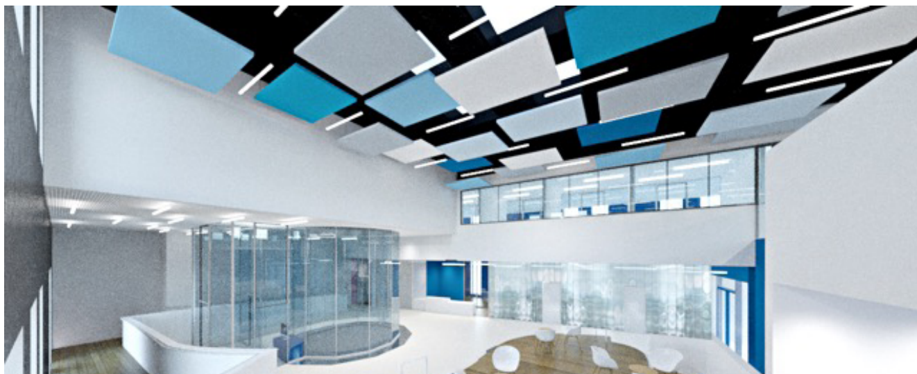
ceiling elements with the purpose of reducing the noise
